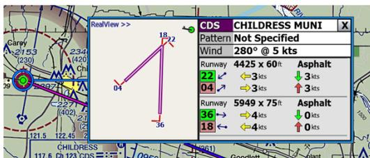
displays the downwind and crosswind component for each runway, color-coded to help the pilot make a quick decision.
